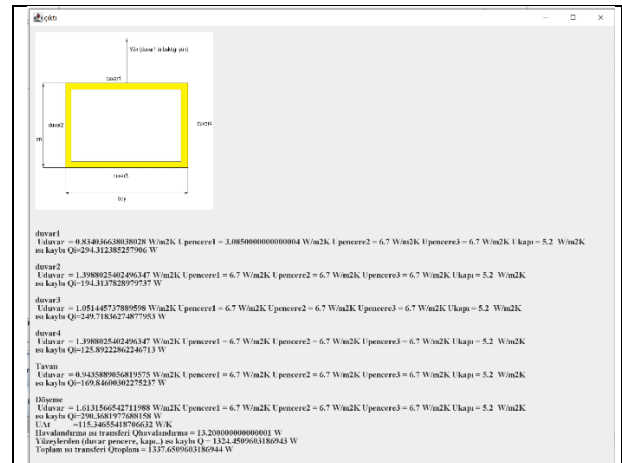
Figure 9. An output GUI window wall design & selection odaP2_2022 (Room heat loss values)
