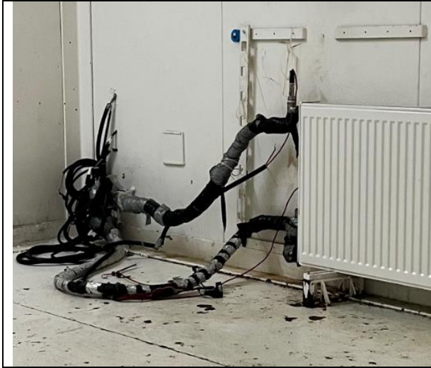
Figure 1. ECA ELBA Radiator heat capacity measurement system
