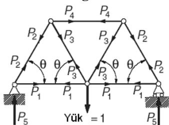
Load Matrix of the figure can be given with the following system of equations
