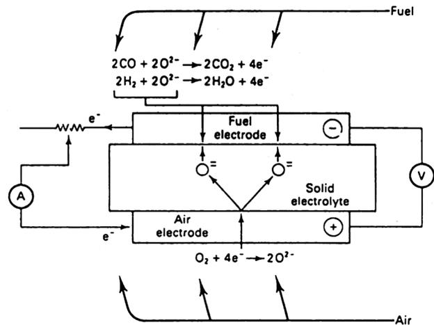
**Fig. 1 Principle of operation of SOFC [5]****Table 3 Some properties of logistic fuel NATO F-76 [9]**
