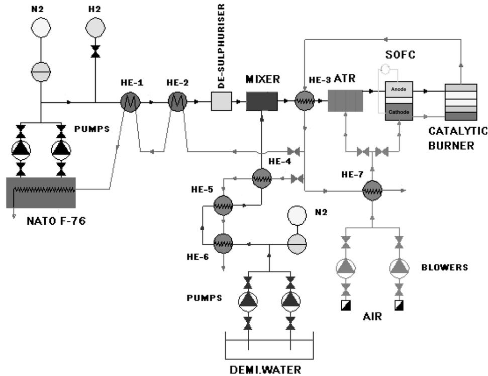
Fig. 3 F-76 diesel-fueled SOFC system auxiliary power unit
