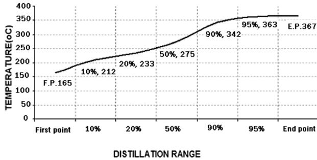
Fig. 2 A typical of distillation curve of NATO F-76
