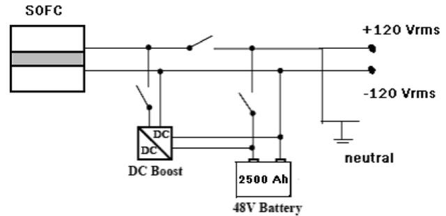
**Fig. 4 Power conditioning for SOFC electric power output**
